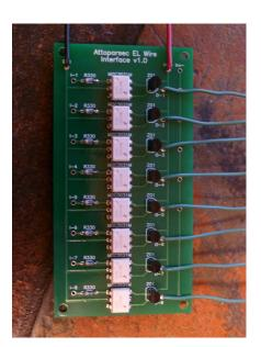
What, you might be asking, can the Attoparsec EL Wire Interface do for you? It can switch up to eight channels of EL wire (or any other high frequency, low power AC) using TTL level inputs. It is ideal for controlling moderately complicated EL wire displays from a microcontroller such as an Arduino. If you are of the bent, you could skip the microcontroller and hard wire a component sequencer, say a simple little 555 + binary counter circuit. The possibilities are only somewhat bounded!
