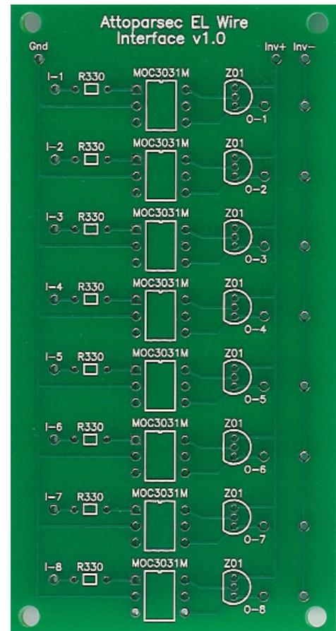
The interface board has 3 global inputs and outputs (**gnd**, **inv+** and **inv-**) and 3 local ones for each circuit (**I-n**, **O-n**, **inv-**).
