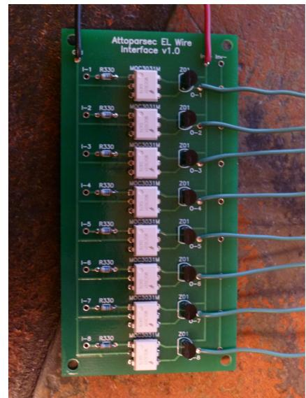
What, you might be asking, can the Attoparsec EL Wire Interface do for you? It can switch up to eight channels of EL wire (or any other high frequency, low power AC) using TTL level inputs. It is ideal for controlling moderately complicated EL wire displays from a microcontroller such as an Arduino. If you are of the bent, you could skip the microcontroller and hard wire a component sequencer, say a simple little 555 + binary counter circuit. The possibilities are only somewhat bounded!
